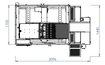
The chassis is totally of stainless steel. AISI-304
